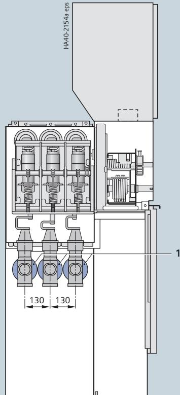
1 Bus/cable-type current transformer 4MC7032
