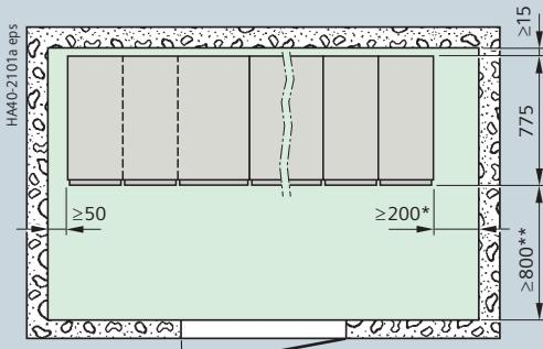
Top view: Switchgear without pressure relief duct at the rear
