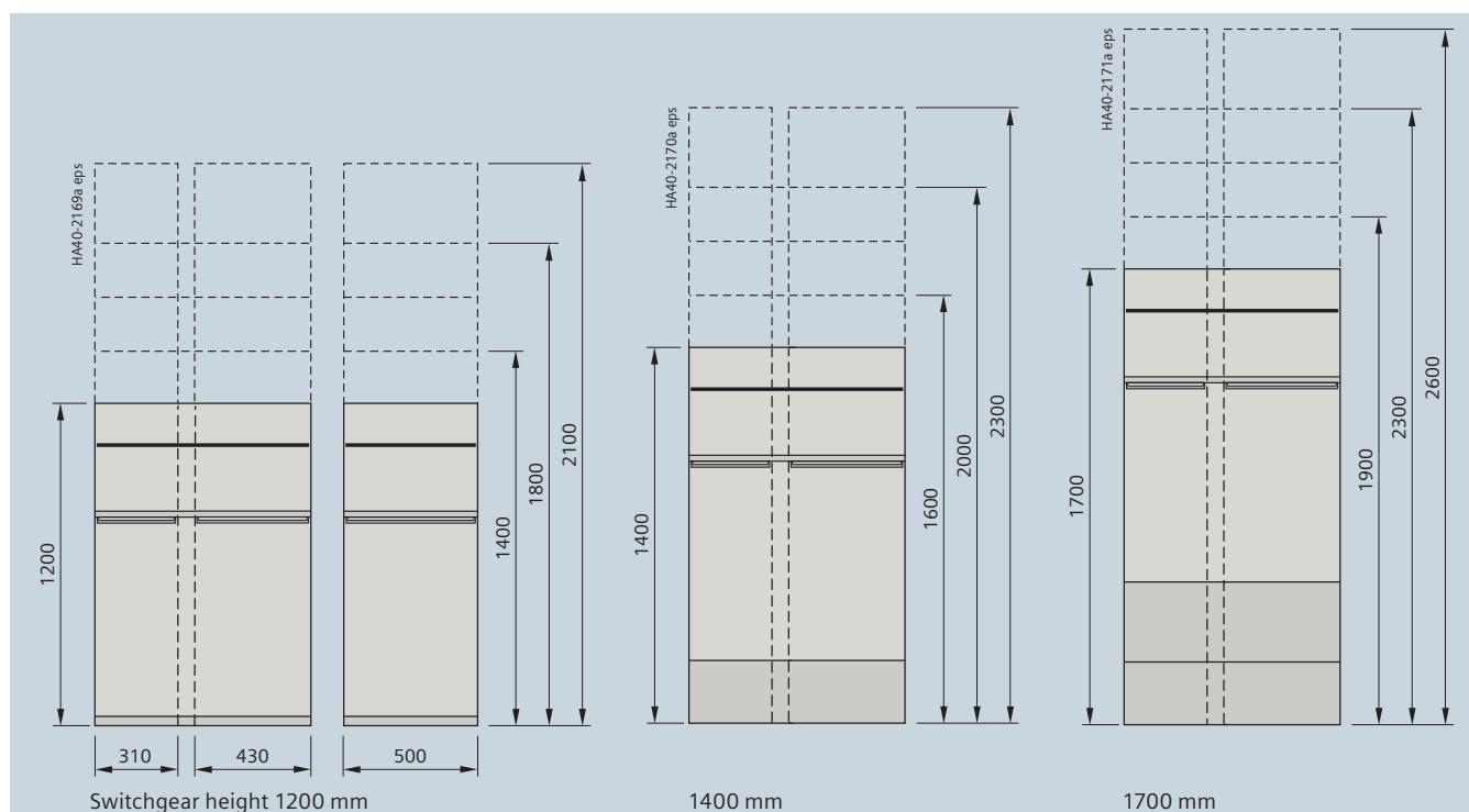
The following type-tested versions of the pressure relief system are available for 8DJH switchgear:
