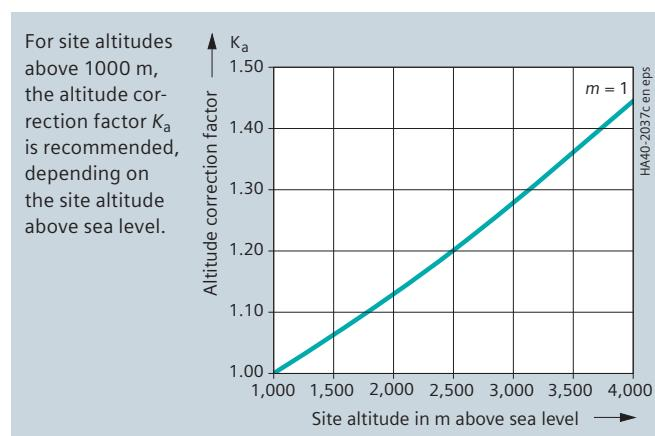
Curve m = 1 for rated short-duration power-frequency withstand voltage and rated lightning impulse withstand voltage according to IEC/EN 62271-1 / VDE 0671-1.
