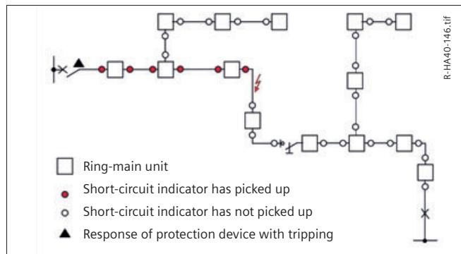
Short-circuit/earth-fault indicators can be used in all kinds of power systems. In impedance-earthed and solidly earthed systems, as well as in isolated and compensated (resonant-earthed) systems, earth-fault detection is also possible.
